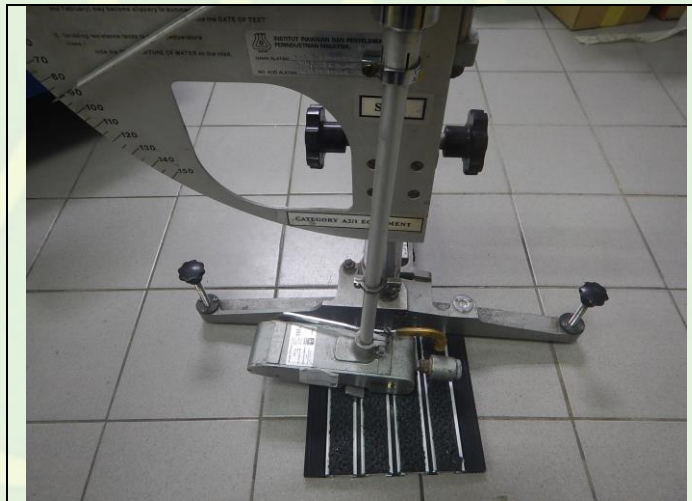
Slip Resistant Test on Wet Condition
